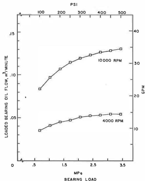
Fig. 9—A comparison of the 4000 and 10 000 rpm shaft speed 100 percent recommended oil flow rates to the loaded bearing for loads that range from 0 to 3.45 MP<sub>a</sub> using an ISO VG 32 lubricant supplied at 46°C.
