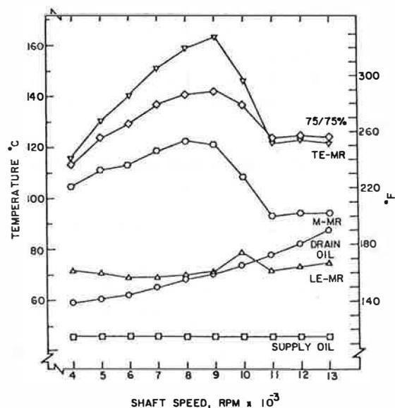
Fig. 4—A comparison of the temperatures recorded at selected locations for a bearing operating at a load of 3.45 MPa for shaft speeds that ranged from 4 to 13 000 rpm using a lubricant supplied at 100 percent of recommended flow rates at a temperature of 46°C.
