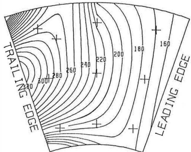
Fig. 2—Bearing pad isotherm showing the thermal gradient across the pad at a shaft speed of 10 000 rpm and a load of 3.45 MPa (500 psi) with 100 percent of recommended flow rate. Temperatures shown are in °F.
