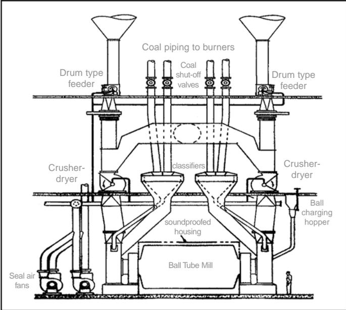
Figure 10. Ball Tube Mill System.
