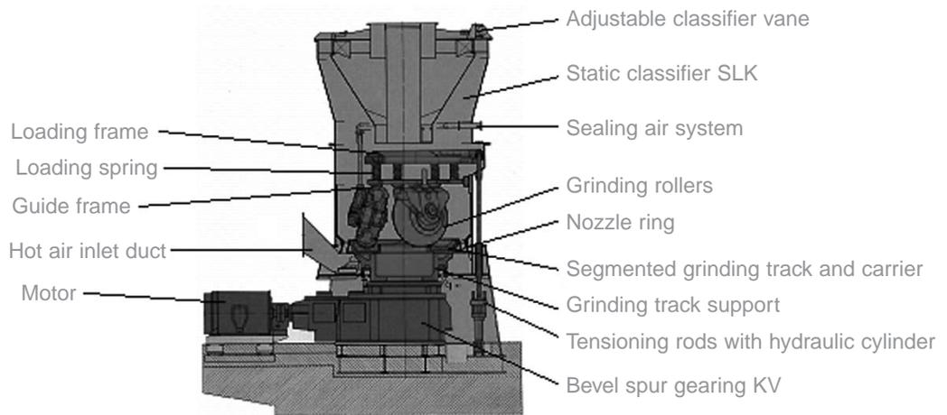
Figure 2. First Generation MPS Mill with spring grinding force loading system.
