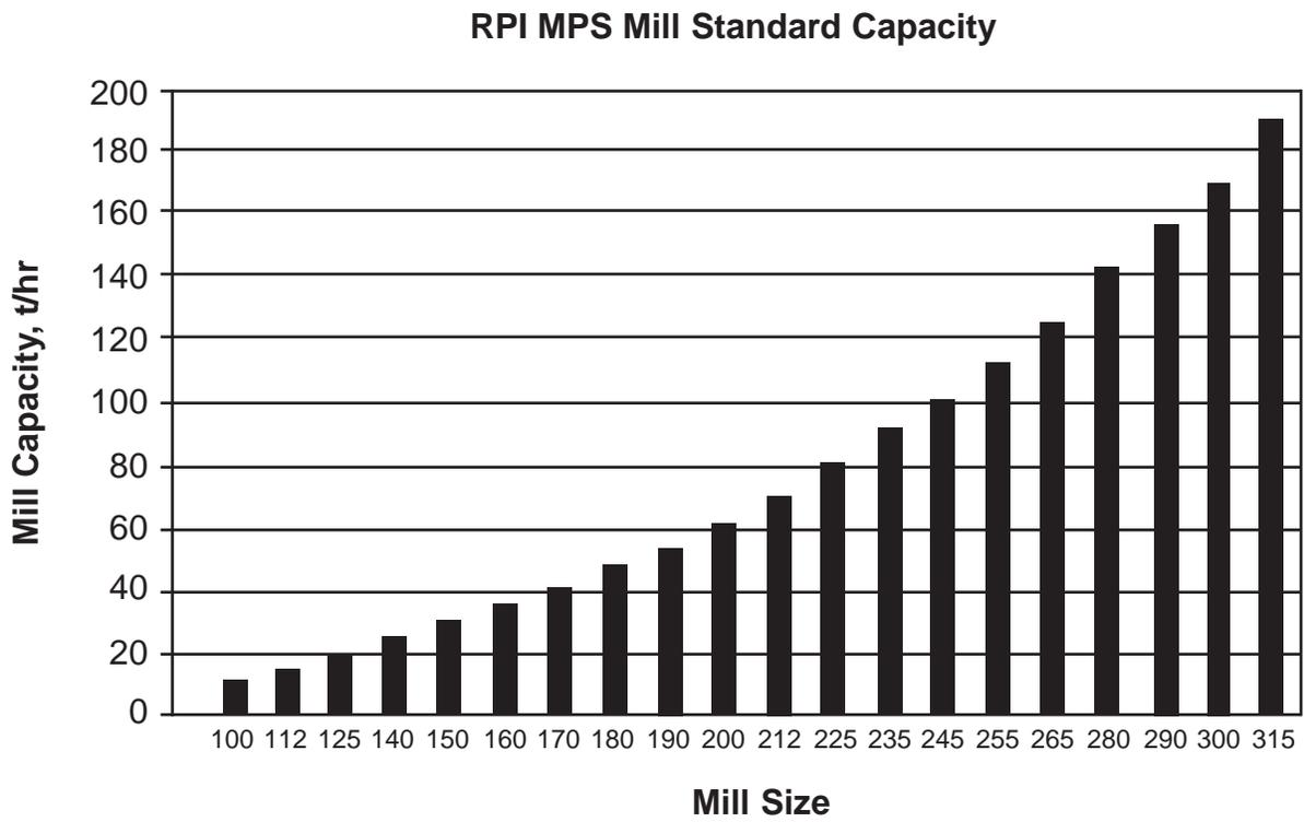
Figure 3. MPS Mill standard capacity.
