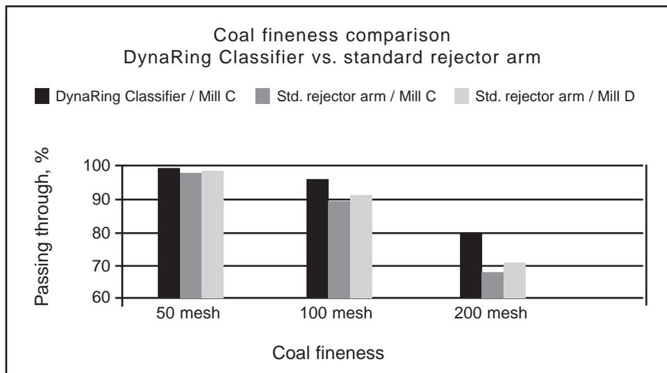
Figure 9. Test Results of DynaRing™ vs. Rejector Arm Classifier.
