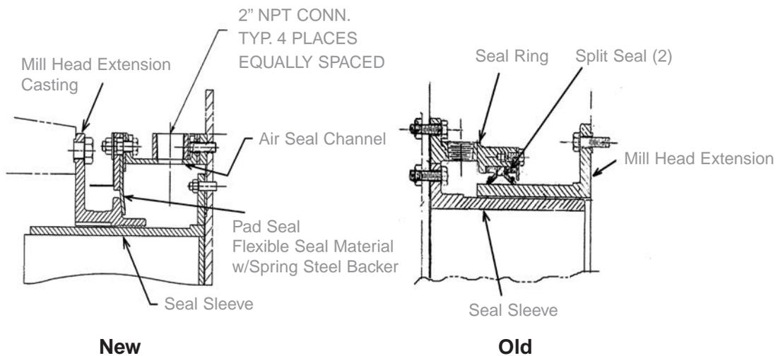
Figure 12. BTM Trunnion Seal Design: New vs. Old.
