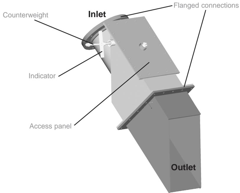
Figure 11. New Trickle Valve Design for BTM.
