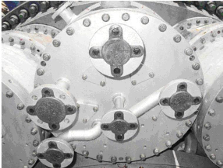
**Figure 11. FME Covers On A Combustion Can End-Cover**
