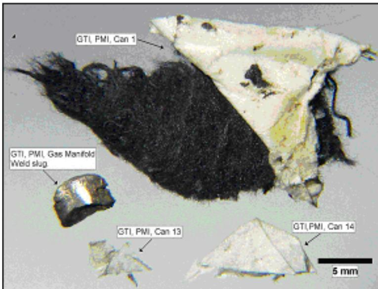
**Figure 10. Example Contaminants found in Gas Piping**
