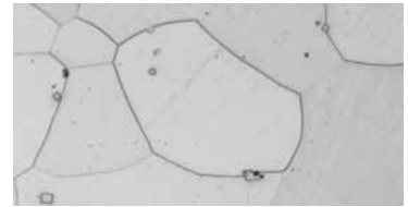
Ferrite (α-iron). Body centered cubic with 8 atom neighbours. 68% packing.
