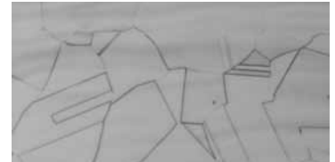
Austenite (γ-iron). Face centered cubic with 12 atom neighbours. 74% close packing.
