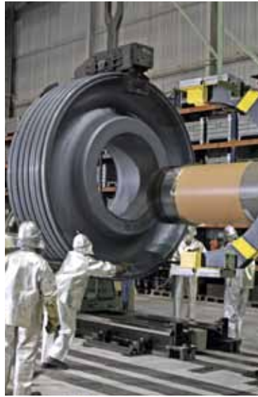
Assembling heated-up disk onto rotor
