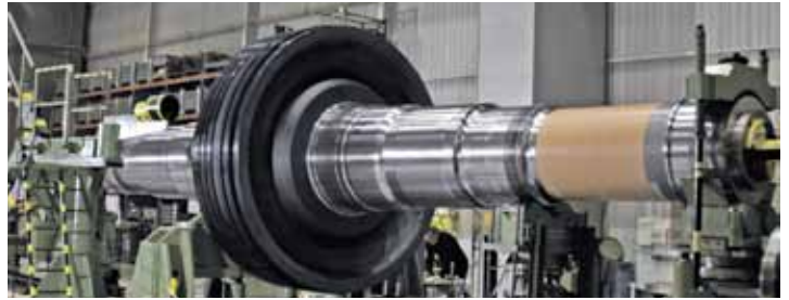
Shrink fit by cooling down of disk on turning rotor
