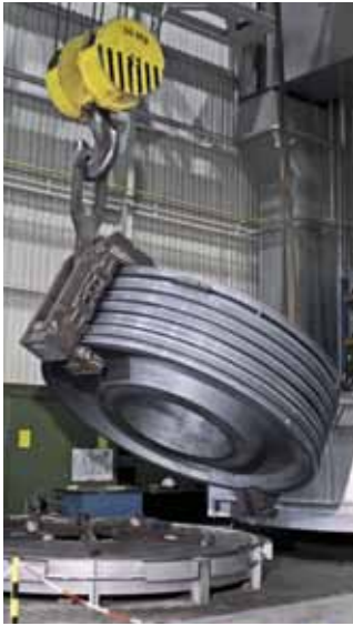
Crane transport of heated-up disk
